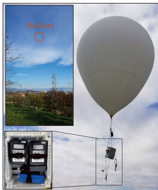
Figure S2. Sampling balloon with the instrumentation.
