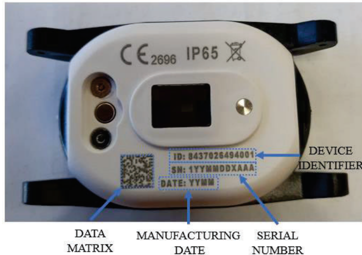
Figure 5.9. Traceability symbols engraved on the ONAVITAL case.
