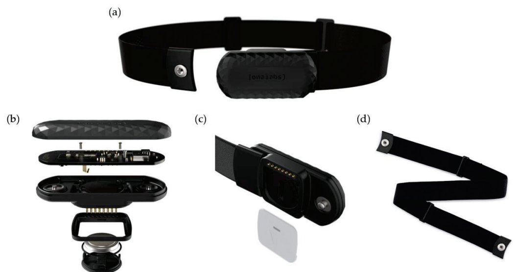
Figure 1. Structure of the wearable device. (a) Complete system, (b) central module (electronics of the system), (c) cartridge, and (d) chest strap.
