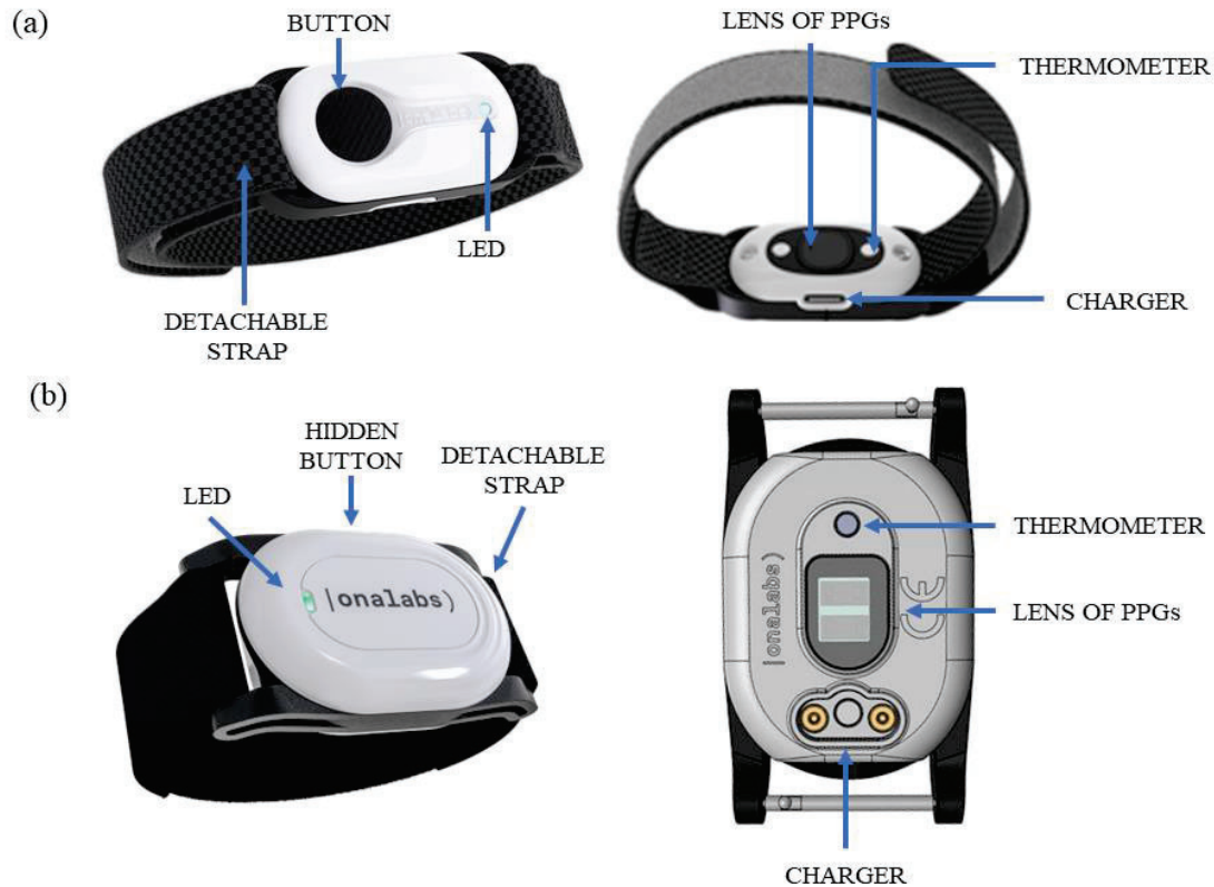
Figure 4.1. Versions of the ONAVITAL device. (a) Device used on the first and the second phase. Courtesy of Aguilar-Torán (2022) [2], used with permission. (b) Wearable device utilized in the third phase.
