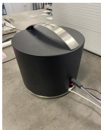
Figure 3. Setup for measuring thermal conductivity of the liquid eutectic sample, covered with an insulating lid.
