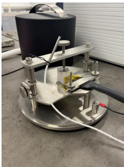
Figure 4. Setup for measuring thermal conductivity of the solid eutectic samples.
