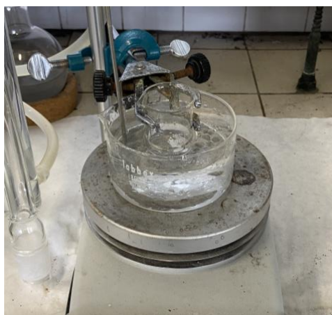
Figure 1. Melting and stirring of the fatty acid eutectic mixture in a water bath on a hot plate.
