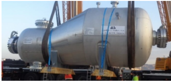
Figure S. Heat exchanger (Photo from Aguilar y Salas) [61]
