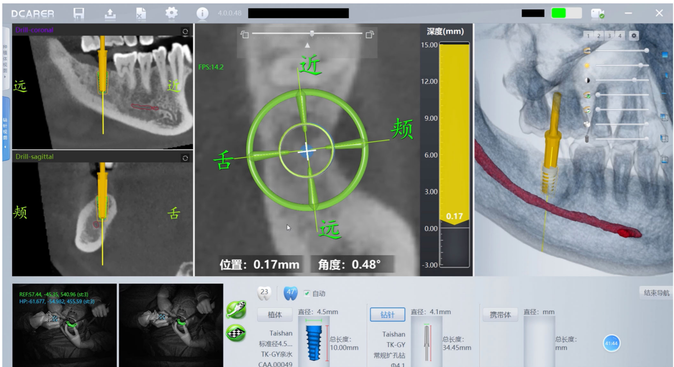
FIGURE 2 | Real-time guidance displayed on the computer screen of the prototype dCAIS system.
