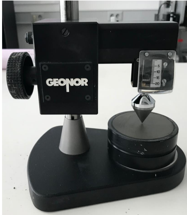
Figure 3.11: Norwegian fall cone apparatus used in this study.
