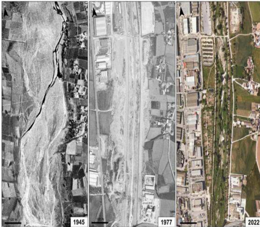
Figure 8. Evolution of the river channel at Granollers from 1945 (left) to 2022 (right). The river channel has been reduced from 300 m wide in 1945 to 80 m in 2022.
