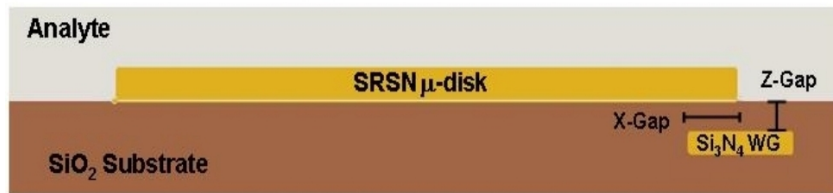
Figure 3.15: Scheme of the cross section of the coupled structure. The Z-Gap and X-Gap are also graphically defined.
