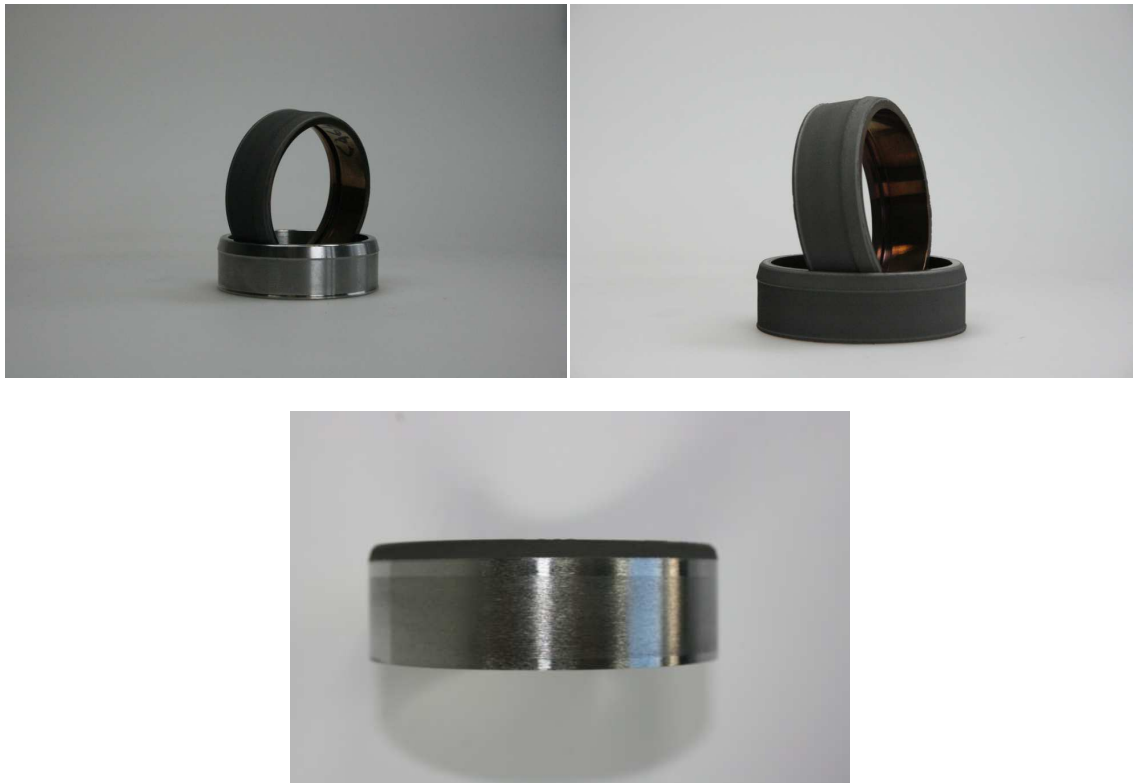
Figure 42. Specific automotive parts before (left) and after (right) coating by CGS; and after machining (down).
