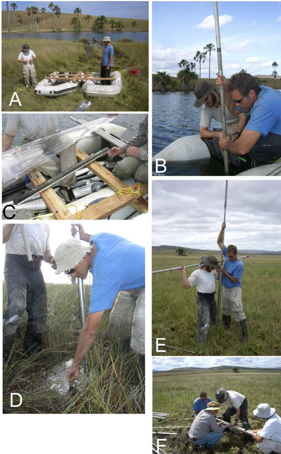
Figure I.6. Core sampling during PATAM 2007 field trip. A-C: Lake sampling with modified Livingston squared-rod piston. D-F: Peat bog sampling with Livingston squared-rod piston. (Photos: E. Montoya, 2007).
