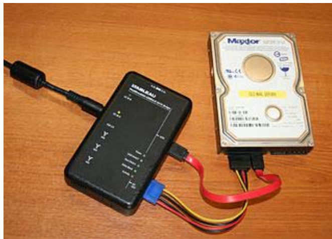
Figura 68. Disc dur (Maxtor) connectat a un write-blocker (Tableau)
