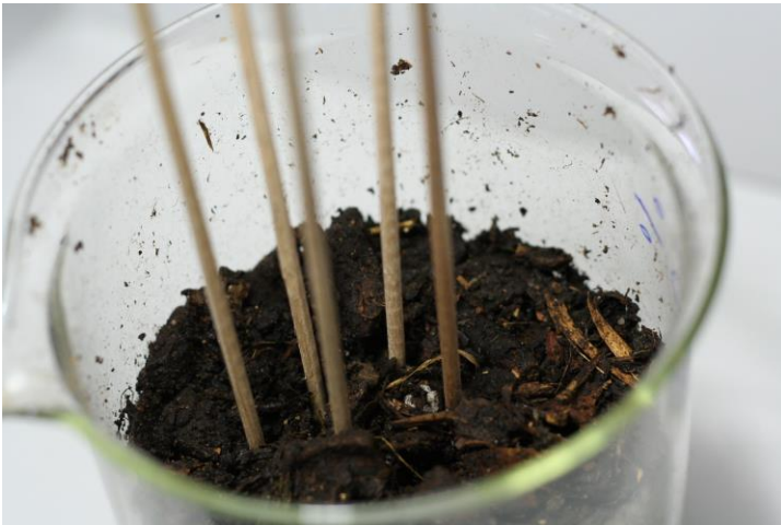
Figure 10. Skewers stuck into the compost for the minimum contact time experiment.
