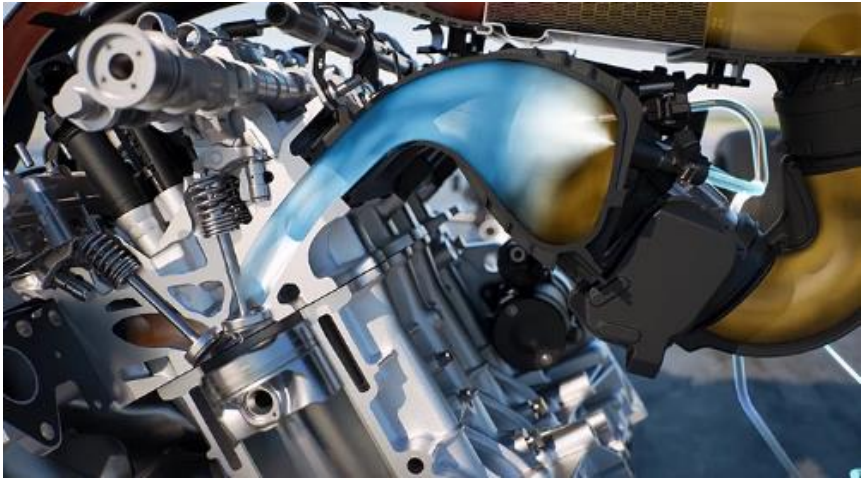
Figure 5: BMW M4 GTS water-injection system. (BMW, 2015)
