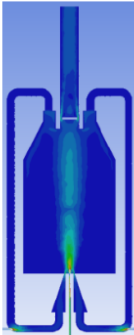
Figure 2: Velocity profiles for the MILD combustor. (Noor et al, 2013)
