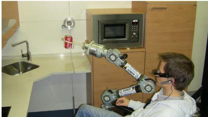
Figure 8. The robot “Grab a red can from a table” task achievement
