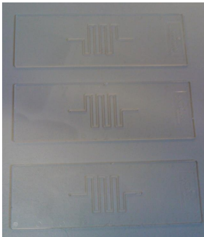
Figure 3.36: New PCR block with loop channel like PCR chamber
