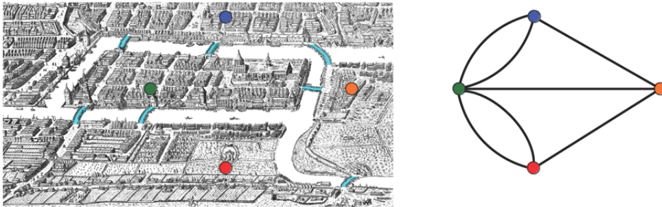
Figure 1.1: The city of Königsberg with its seven bridges. In 1735 Euler used a network representation to prove that there was no route that crossed each of the seven bridges of the city of Königsberg only once.
