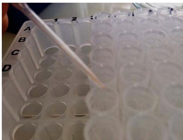
Figure 91: Orange-reddish dyed pipette tip after performing dilutions without changing the tips.
