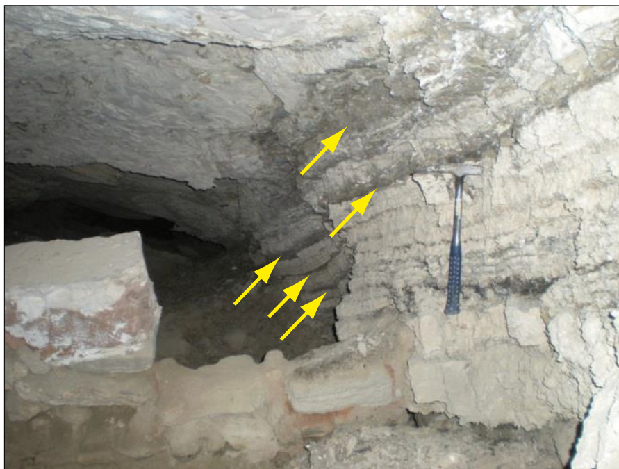
FIGURE 9. The samples collected from an old sulfur mine in the Cenajo Basin (CMM) with a TOC content up to 14 % and S 2 up to 100mg HC/g rock. Arrows indicate organic-rich levels interbedded with gypsum.
