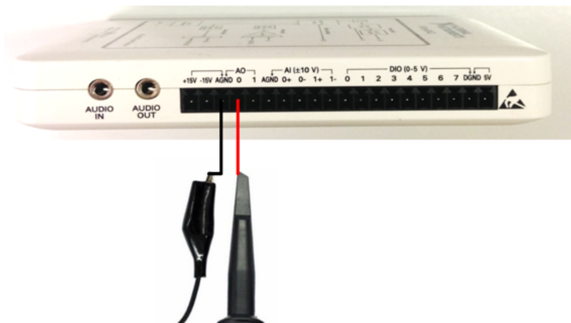
Figure 23 Connection of the Oscilloscope probe to Protoboard
