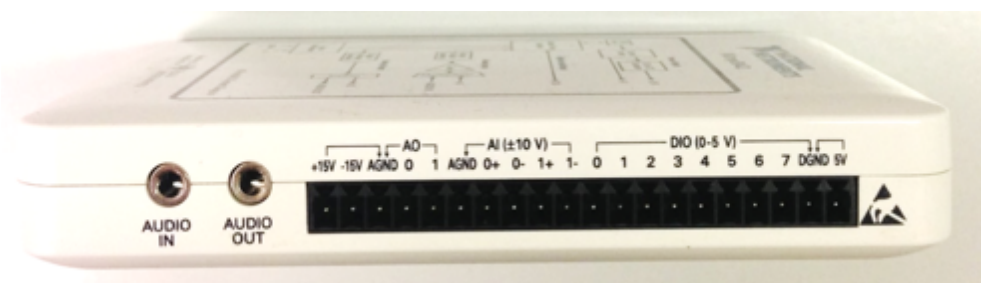
Figure 2 Input and Output ports of myDAQ
