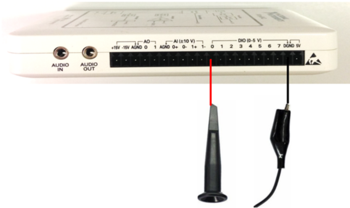
Figure 36 Connection of the oscilloscope probe to protoboard
