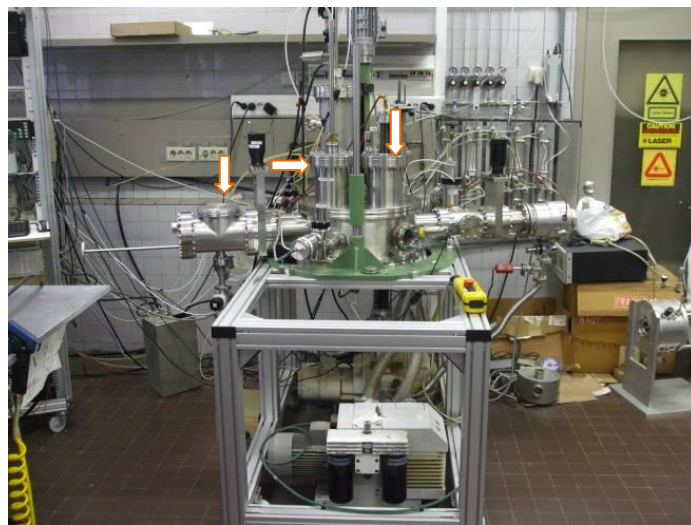
Fig. 12. Reactor: From left to right; place to introduce sample inside the chamber and 4 different heads; 2 for Fe and Si sputtering, 1 for heater and PECVD reaction and last one is free.
