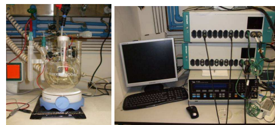
Fig. 6. a) Three electrode e-cell system b) AutoLab System
