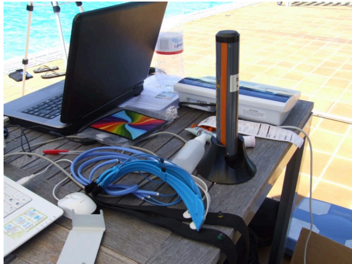
Figure 8. Waterproof heart rate Freelap monitors and bacons for the recording of heart rate and swimming time laps, time, and speed.
