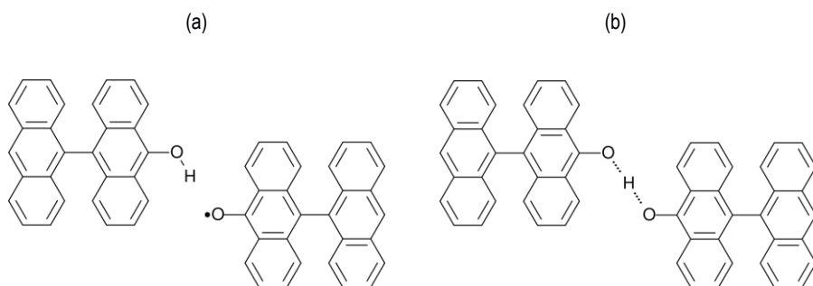
Figure 4. Anthranol/anthroxy radical pair schematic structures. (a): structure at 100K, (b): structure at 200K
