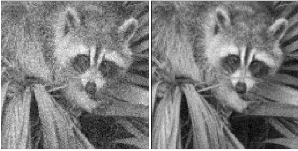
SSIM: 0.69 16,000/16,384 Matrices SSIM: 0.87 16,300/16,384 Matrices FIG. 7: Images of 128x128 pixels with their SSIM and number of matrices used. It is clearly seen how the quality of the image improves.
