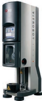
Figure 3.3 FEI Vitrobot. Used for sample vitrification. (Taken from Web 3 .)
