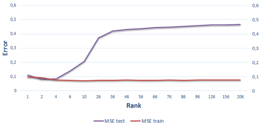
Figure 8: Training and testing MSE trend of PBRs using the scoring function S2 and the parameter Set 2.
