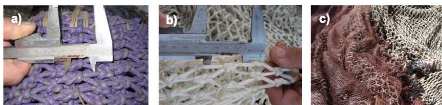
Figure 5. Pictures of the two mesh sizes tested for selectivity: a) 50 mm diamond and b) 40 mm square mesh. c) shows the codend covered with a 3 mm mesh size net in order to determine selectivity of the gear
