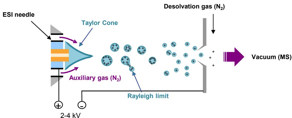
**Figure 1.14:** Schematic representation of the basics of spray formation in electrospray ionization (ESI).
