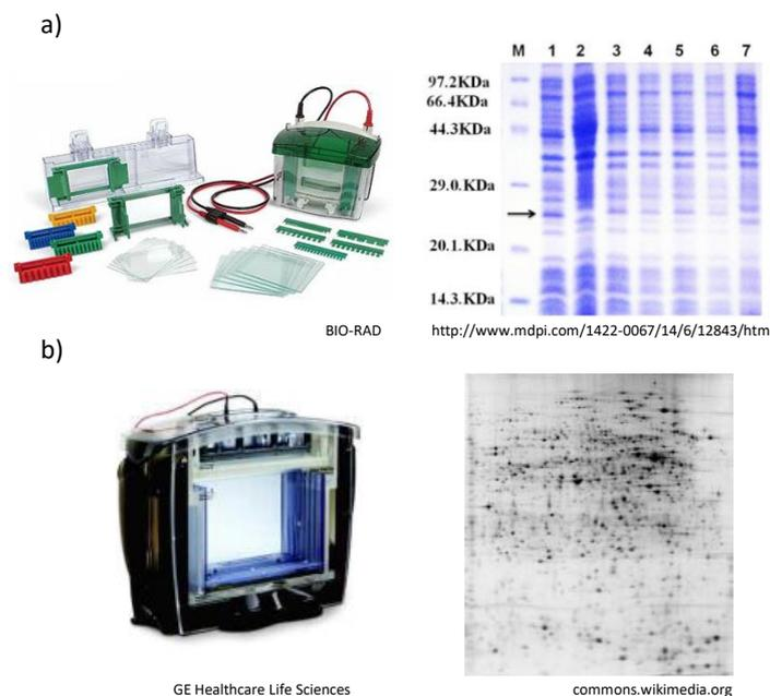
**Figure 1.18:** Typical instrumentation and obtained gel with a) polyacrylamide gel electrophoresis (SDS-PAGE) and b) two-dimensional polyacrylamide gel electrophoresis (2D-PAGE).
