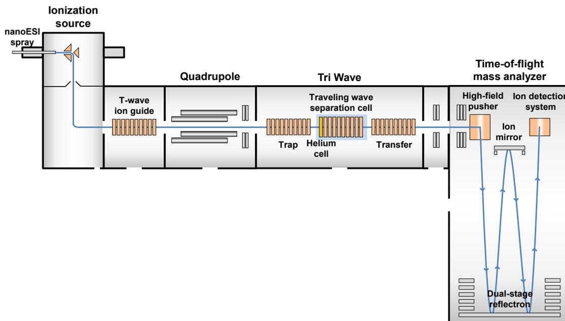
**Figure 1.17:** Schematic representation of an ion mobility mass spectrometer (IM-MS) with a traveling wave ion mobility cell (Synapt G2 from WATERS® Corp.).
