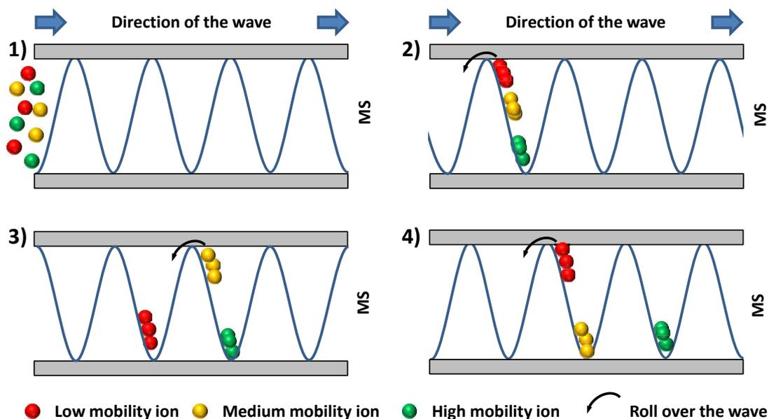
**Figure 1.16:** Fundamentals of TWIMS separation. High mobility ions travel with the wave, thus, arriving first to the MS. Whereas, low mobility ions roll over the wave, spending more time in the mobility cell and, therefore, arriving later to the MS.
