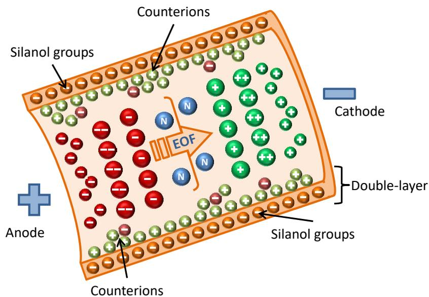
**Figure 1.19:** Differential ion migration depending on charge and size due to the electroosmotic flow (EOF) in capillary electrophoresis (CE).
