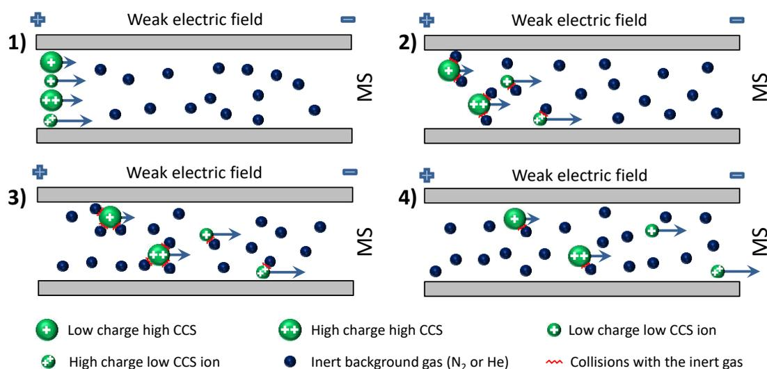
**Figure 1.15:** Separation in classical IM-MS. Ions with smaller CCS and higher charge are separated before those with higher CCS and smaller charge.
