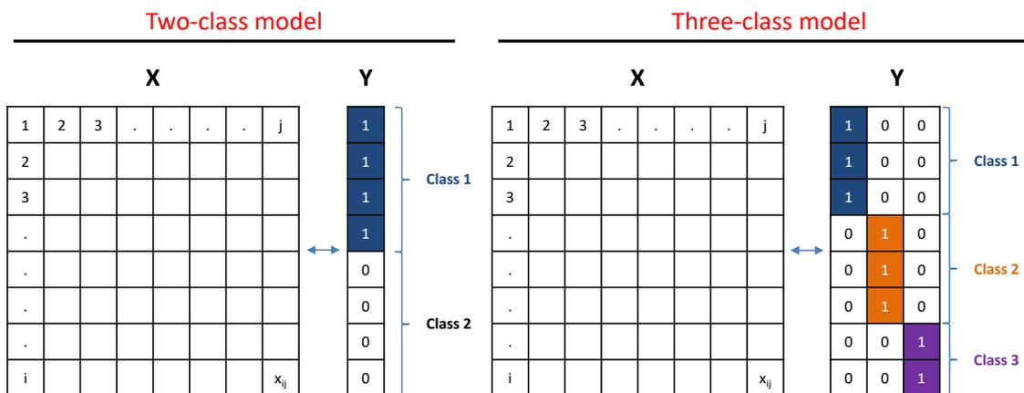
**Figure 1.21:** Representation of partial least squares-discriminant analysis (PLS-DA) for models including two classes and three classes.
