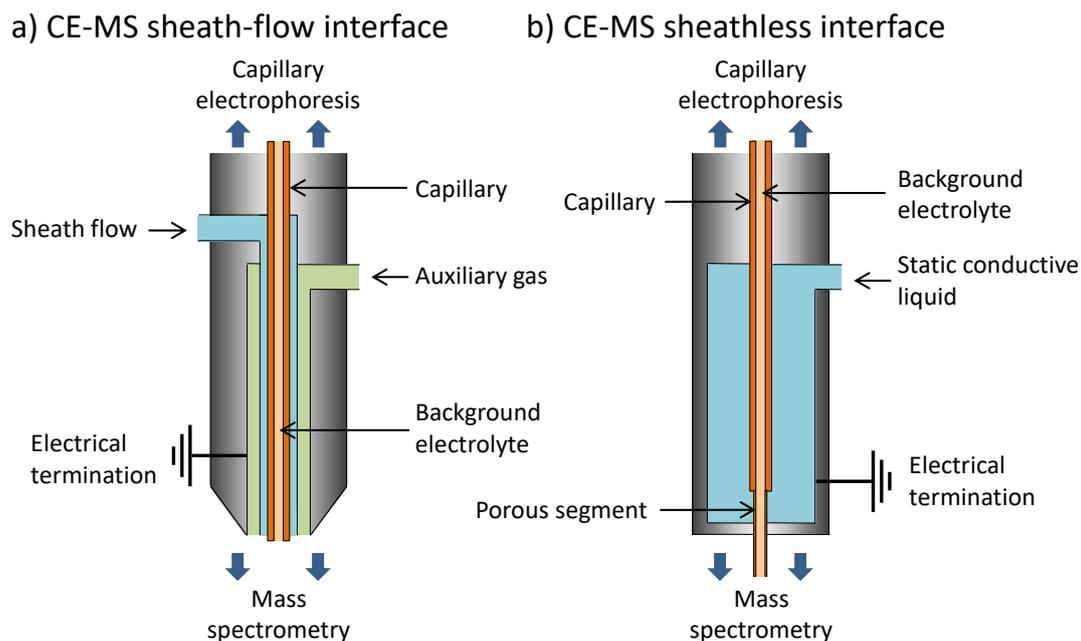
**Figure 1.20:** Schematic representation of the a) sheath-flow and b) sheathless interface for coupling capillary electrophoresis to mass spectrometry.
