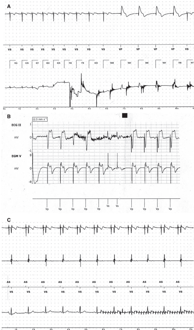
Fig. 2. Examples of normal pacemaker function despite noise in the electrocardiogram recordings. (A) During ultrasonic dental scaler testing in a patient with atrial fibrillation, noise in the electrocardiogram is detected without affecting normal ventricular pacing in the case of slow conduction. Tracings from top to bottom: ventricular channel, device markers, surface electrocardiogram. (B) Normal ventricular pacing and ventricular sensing despite electrocardiogram noise during electric pulp tester testing. Tracings from top to bottom: surface electrocardiogram, ventricular channel, device markers. (C) Normal atrial and ventricular sensing during electric pulp tester testing despite electrocardiogram noise. Tracings from top to bottom: atrial channel, ventricular channel, device markers, surface electrocardiogram.
