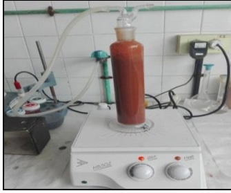
Figure 3.4: Experimental procedure of leaching of Gossan ore by cyanidation
