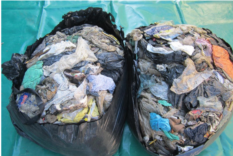
Figure 12. Initial sample of the rejection from a biological-mechanical treatment plant of solid urban waste
