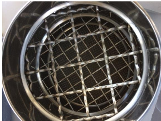
Figure 5. Vibrational sieve with sieves of 200 mm of diameter with the following mesh openings: 1.8mm, 2.8mm, 2cm and 4cm.
