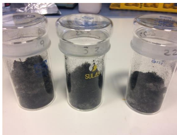
Figure 10. Prepared sample for the analysis of moisture and elemental analysis of tire rejection.
