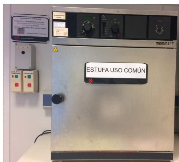
Figure 11. Electric oven for the determination of moisture, volatile content and ash content.
