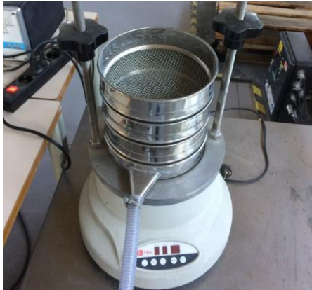
Figure 5. Vibrational sieve with sieves of 200 mm of diameter with the following mesh openings: 1.8mm, 2.8mm, 2cm and 4cm.
