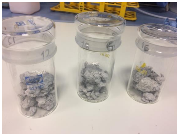
Figure 9. Prepared sample for the analysis of moisture and elemental analysis of sludge from a paper industry.
