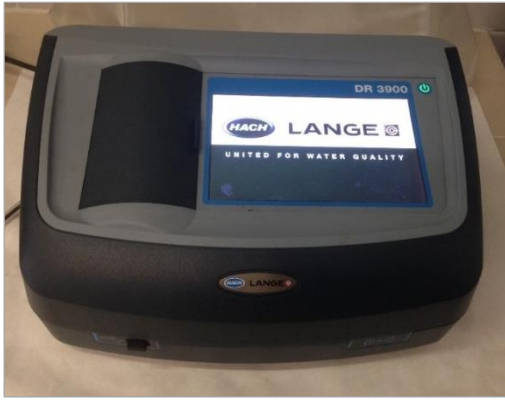
Figure 8: Spectrophotometer Hach Lange DR 3900
