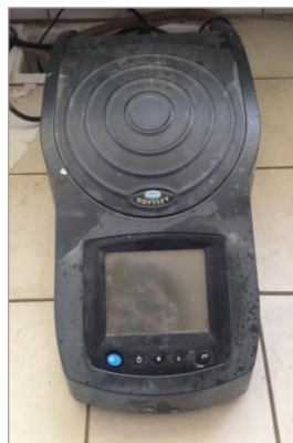
Figure 10: Spectrophotometer Hach Lange DR 6000
