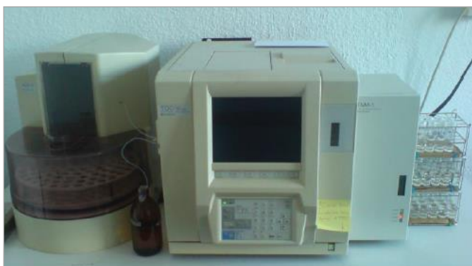
Figure 7: TOC-VCNS analyzer Shimadzu
