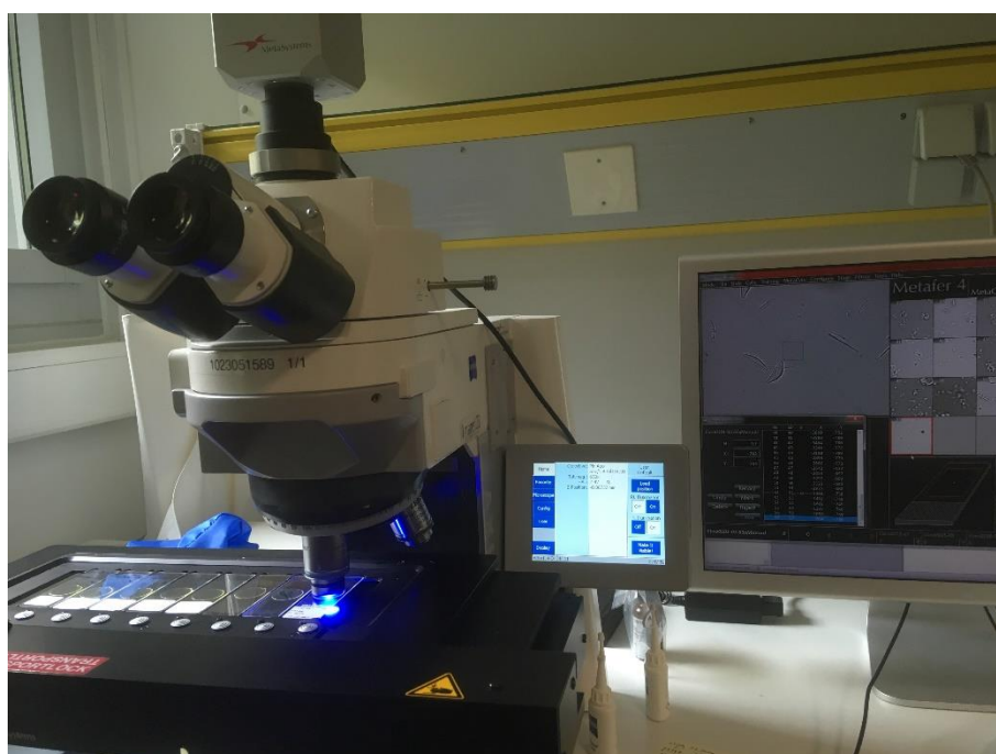
AnnexFigure 8 Zeiss Axio M2 Microscope attached to Metafer system as an automatic slidescanner.
