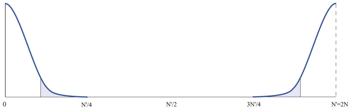
Figure 7.4: New distribution of Fourier coefficients in a double sized grid and in between zeros.
