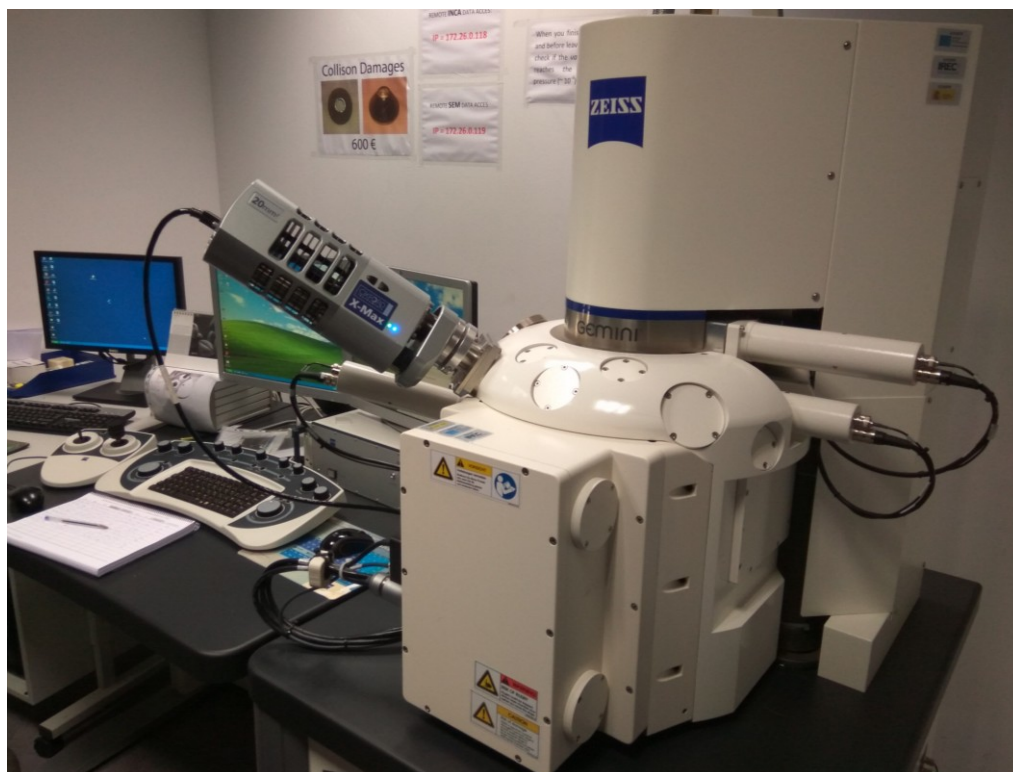
Figure 3.12. – Picture of the scanning electron microscope Zeiss Serie Auriga FESEM.
