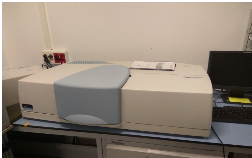
Figure 3.11. – Picture of the UV-visible spectrometer Perkin-Lambda 950.
