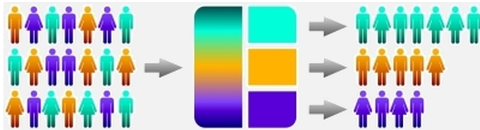
FIGURE 4.1: Collavorative filtering recommends items to a user based on its similar peers' items.
