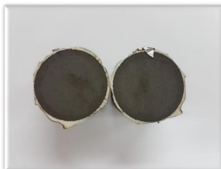
Figure 45: Cohesive failure after tensile strength test
