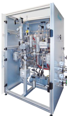
Figure 15. FISCHER apparatus to determinate liquid-vapor equilibrium.
