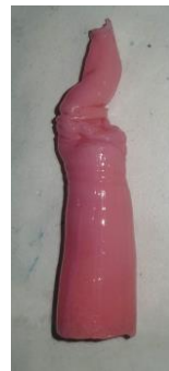
Figure 22. Emulsion gelled - preliminary test.
