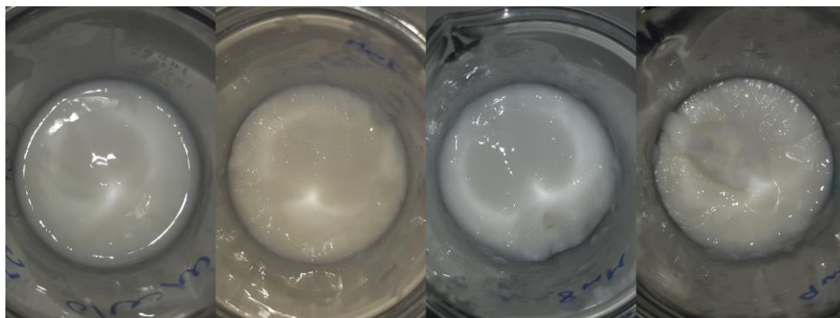
Figure 35. Oil in water in water gelled emulsions at 24 hours. From left to right: emulsions A, B, C and D.
