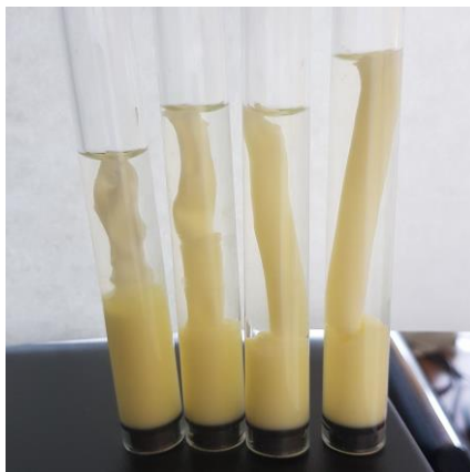
Figure 23. Gelation test with different gelation solutions with mass percentages, from left to right, of 0.25%, 0.50%, 0.75% and 1.00%.
