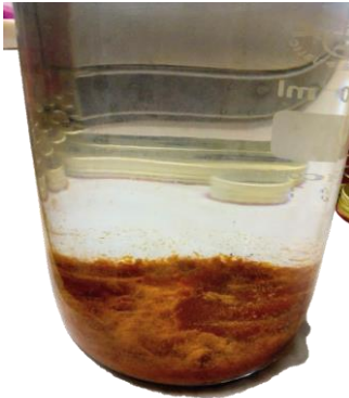
Figure 7. Example of sludge generated by precipitated iron.
