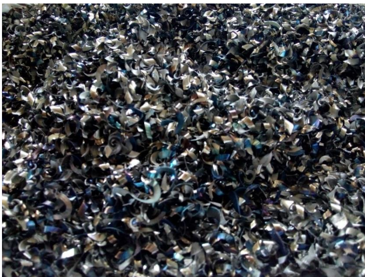
Figure 3. Photo of waste metal shavings ( 0.90\pm 0.45 mm)
