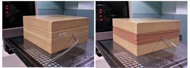
FIG. 1: Homogeneous phantom of water-equivalent material (left) and heterogeneous phantom including a layer of lung-equivalent material (right).
