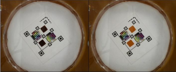
FIG. 6: CO 2 colorimetric sensor printed inside a QR code. Synthetic air pulse picture (left), CO 2 pulse picture (right).
