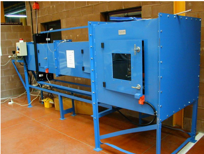
Figure 4.6 Gas canyon used in the experimental trial.
