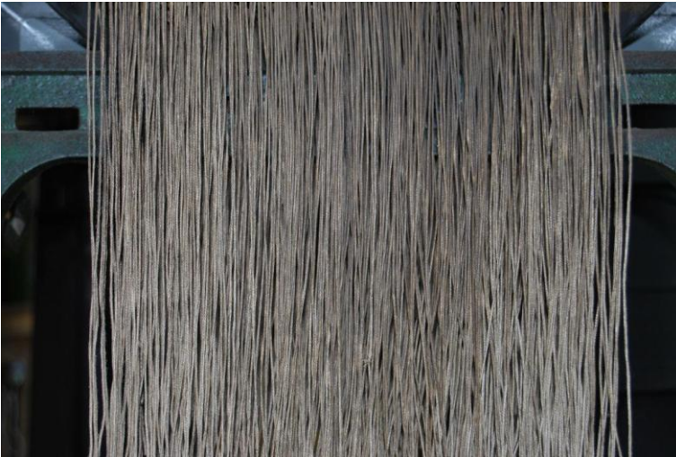
Figure 4.3 Glass fibers produced by a textile machine.
