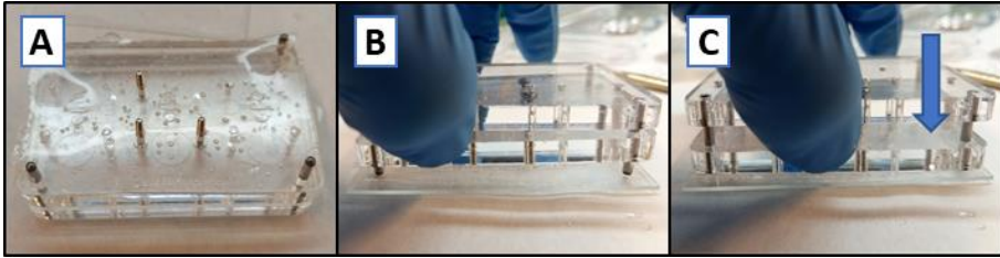
Figure 4-17. PDMS aligning helper. After demolding, the PDMS layer was aligned with the stainless-steel pins (A) and flipped on top of previous PDMS layer, using the pins to align (B). Rigid PMMA layer is finally slid down (C) to bring the surface into contact without misalignment.
