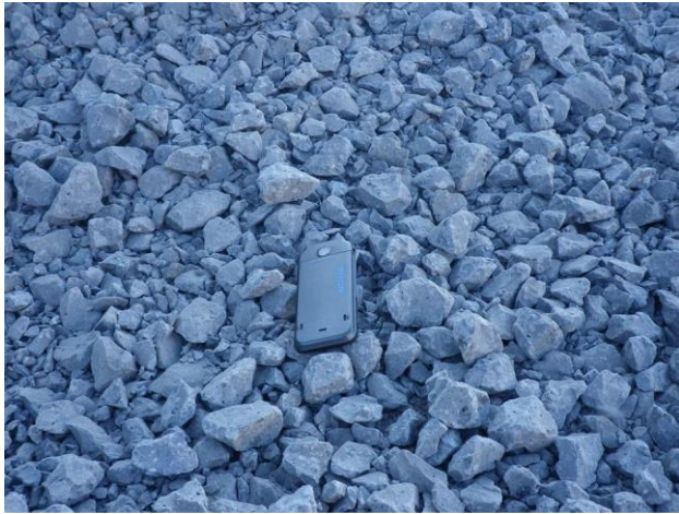
Fig. 1 Crushed hard mortar aspect before mixing with WBA for obtaining the granular material
