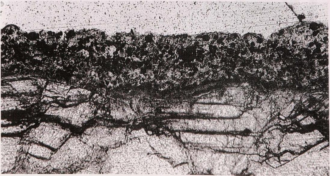
Fig. 7: Gypsum layer on a thin micritic layer. Inside the gypsum layer there are many small, rounded crystals...
