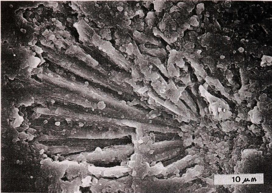
Fig. 11: SEM image of a spherulitic arrangement of calcite crystals around a central micritic nucleus which is rich in P. It corresponds to a microstromatolitic layer developed on granite. Cathedral of Seu d'Urgell.
