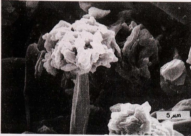
Fig. 8: Gypsum crystals associated to a filament. According to the size and shape of the crystal aggregate it seems to be developed on this filament, suggesting a biological origin for these crystals.
