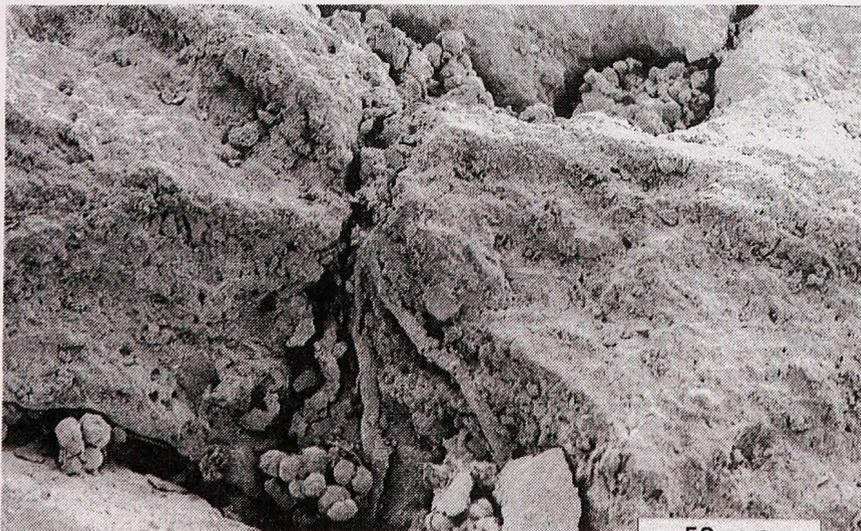
Fig. 10: Orange micritic layer developed on a siliceous sandstone. The patina itself is colonized by black yeast-like fungal colonies (upper part of the photo) which develop hyphae penetrating inside the patina and leading to its decay. The sample corresponds to the Monastery of Sant Cugat del Vallès.
