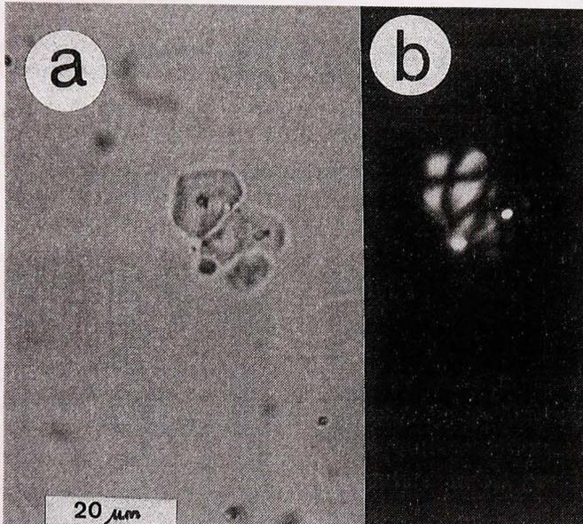
Fig. 9: Small crystals of weddellite (?) accumulated on the surface of the patina. a) polarized light, b) under crossed polars. In the center of each of the crystals a highly birefringent body (a bacteria?) causes a deformation of the crystal structure which is visible by the undulating extinction visible under crossed polars.
