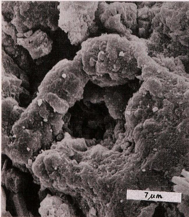
Fig. 12: Mineralization of calcite and Ca-oxalate (?) developed on a filament in the upper part of a patina developed on a calcarenite (Church of Montblanc).
