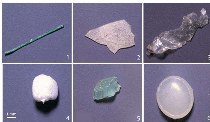
Figure 1.10 Examples of MPLs shapes: 1) line/fibre 2) sheet, 3) film, 4) foam, 5) fragment, and 6) pellet/granule (Wu et al. 2018).
