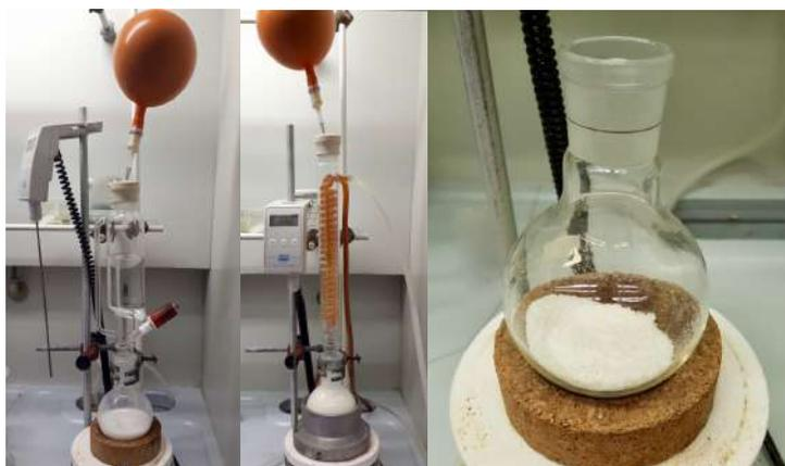
**Figure 2.** Reaction set-up (left), reflux set-up (middle) and final product (right)
