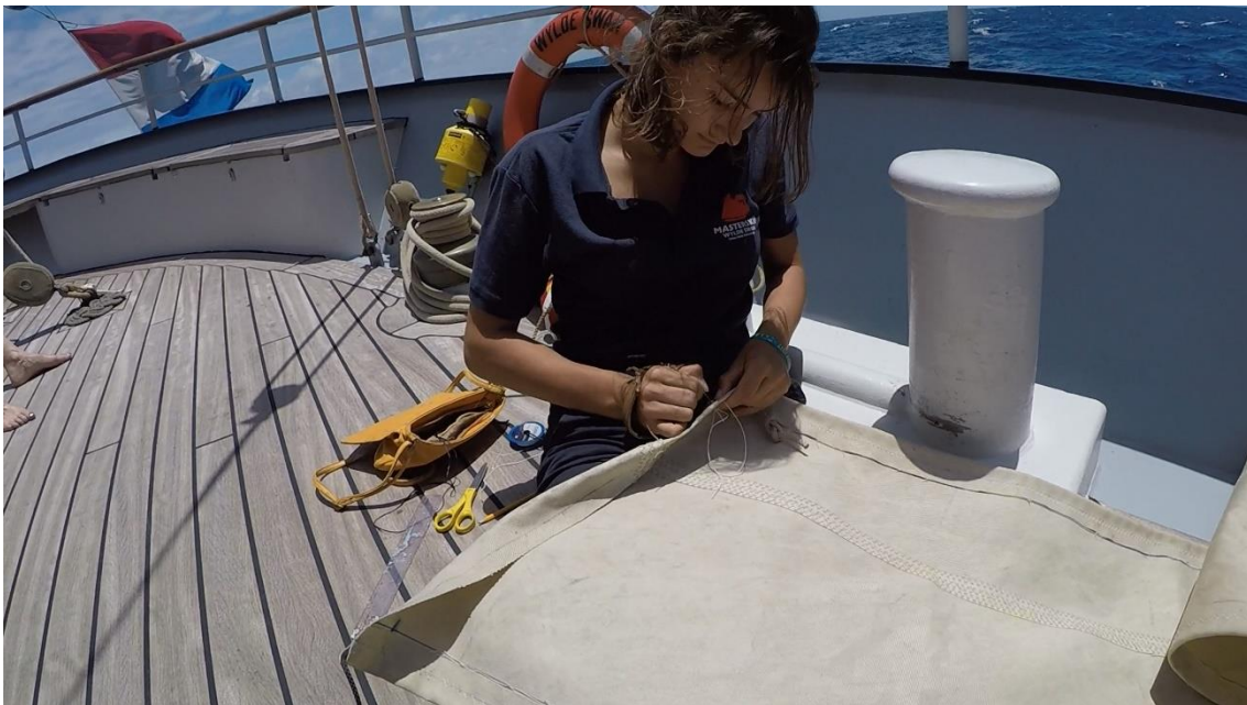
Figure 119: Sewing a piece of sail to make a cover for the base of the mast. She does it with a big needle that is pushed with a leather hand protector – normally called 'Palm' in English, containing a piece of iron inside to push the needle.
