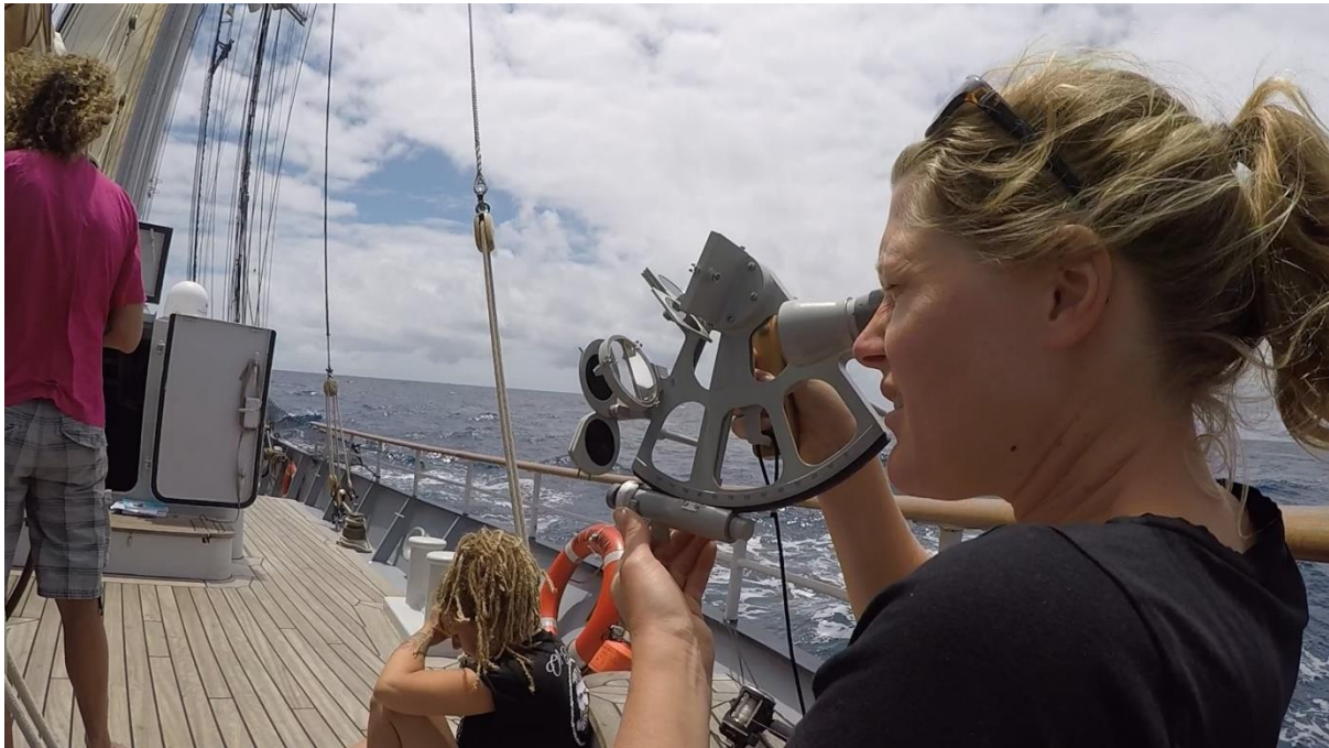
Figure 111: Using the sextant to discover the exact position measuring the angle between the sun and the horizon. Wylde Swan , 2017.
