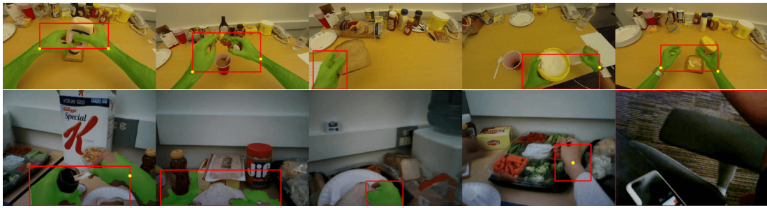
Figure 6.3: Examples of primary regions extraction taken from random frames from the GTEA and GAZE+ datasets. The green-colored regions show detected skin pixels, the yellow dots are the wrist center locations, and the red bounding box shows the located primary region.
